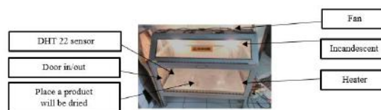
Figure 1. Electric dryer used
