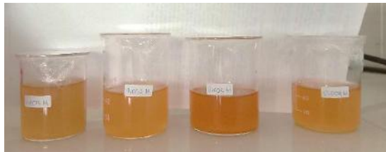
Figure 1. Synthesis result of silver nanoparticle with bioreductor (cempedak bark extract) with concentration level of \text{AgNO}_3 0,0015; 0,002; 0,003; 0,004 M.
